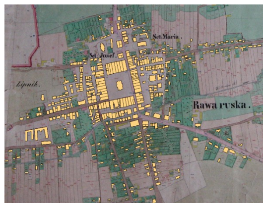
Figure 3: Buildings and houses in Rawa Ruska (shown in beige) after being digitized from the cadastral map and saved in the GIS database.
